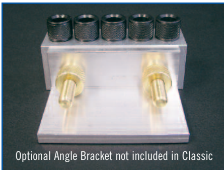
Close-up of T-joint Configuration; for drilling the face portion of a T-joint.
