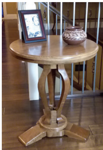
Chess table RIGHT Side table, 80% dowel construction
